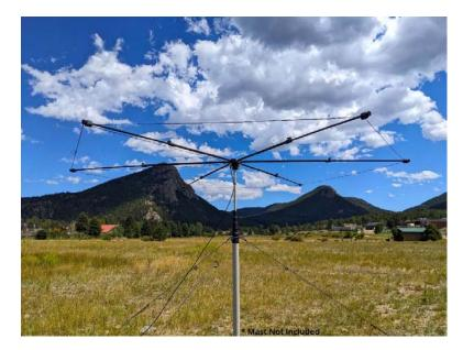
E. Attach Cord in location as shown in "Sketch 1" by looping the ends over the tip of the spreader arms.
